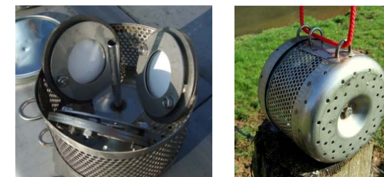
POCIS-Membranes in a triplecate setup. Right: closed exposure cage.
